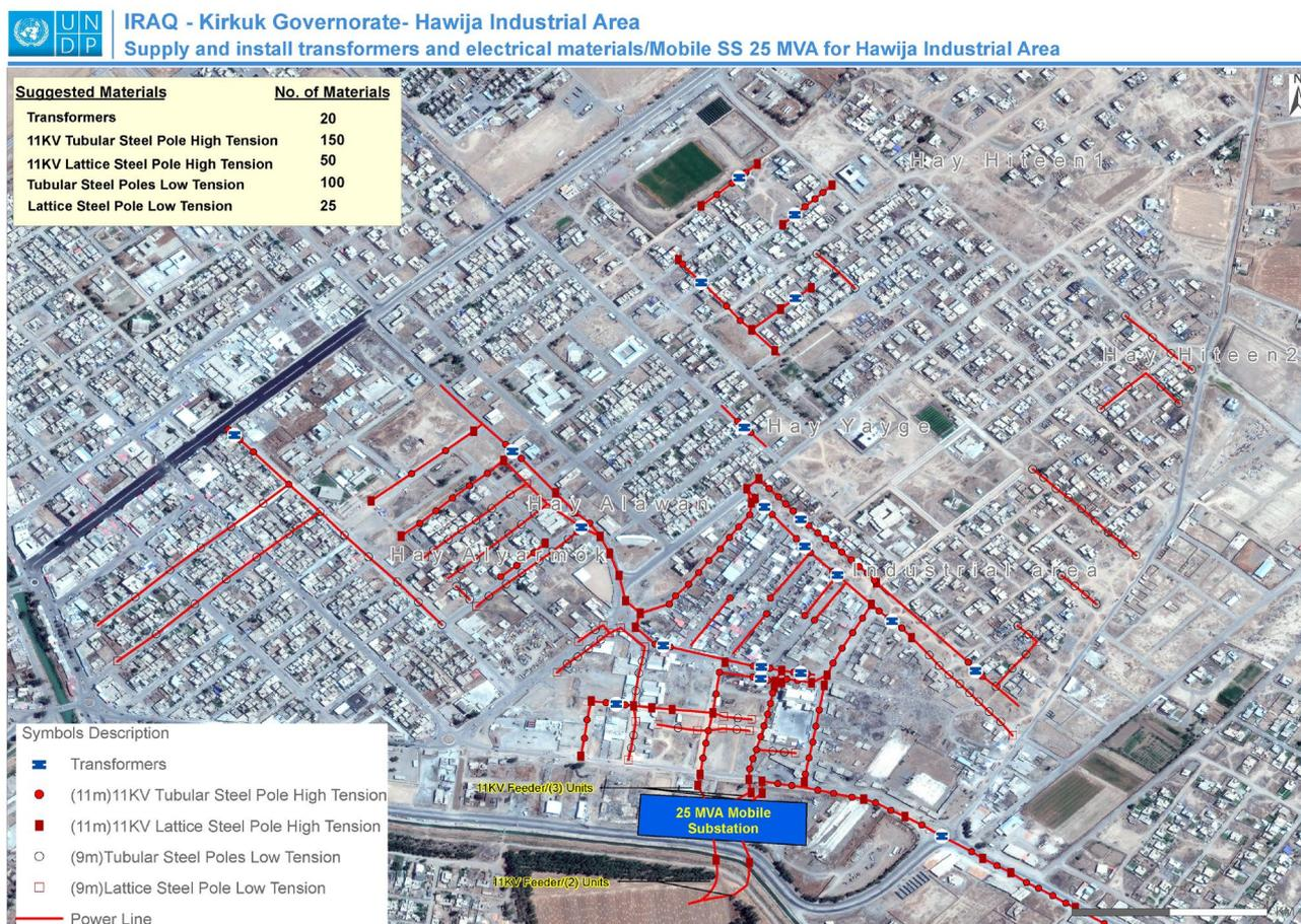
**Electrical distribution network with the location of the installed electricity poles.**
